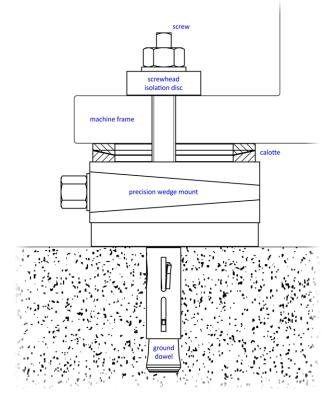
As described above, height adjustment is facilitated starting from the top-most levelling height, proceeding downwards.
